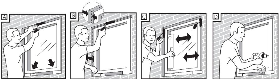
1. Place the window frame inside the wall cave and observe in and out position (fig. A).
